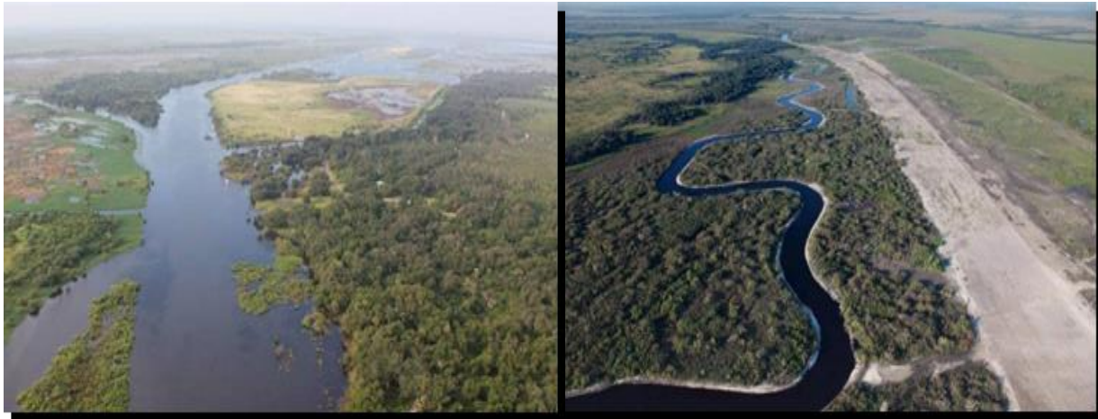
Figure C: Before and after backfilling of the C-38 canal in the Kissimmee River.
